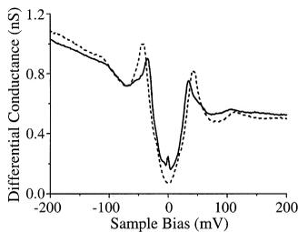
Fig. 2. Tunneling conductance versus sample bias taken at two different locations on the BSCCO crystal. The dashed line is taken on a ‘regular’ superconducting region, where QPSRs are absent. The solid line is a typical spectrum taken at the center of a QPSR, exhibiting a low-energy resonance peak.
