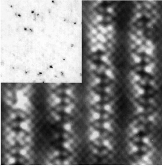
Fig. 1. Typical constant current topograph (10 nm square), showing both atomic resolution and the supermodulation. Inset: A 50 nm square zero-bias conductance map. The QPSRs appear as  $\sim 3$  nm diameter dark regions, owing to their higher zero bias conductance.
